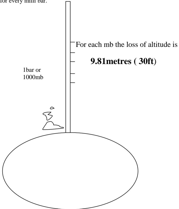
Using the standard we can calculate the pressure loss, due to altitude .
