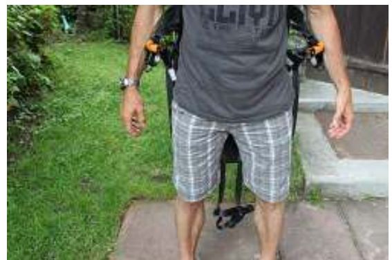
Picture 2: With this type of harness, a take off with open latches/straps, as shown, is almost impossible.
