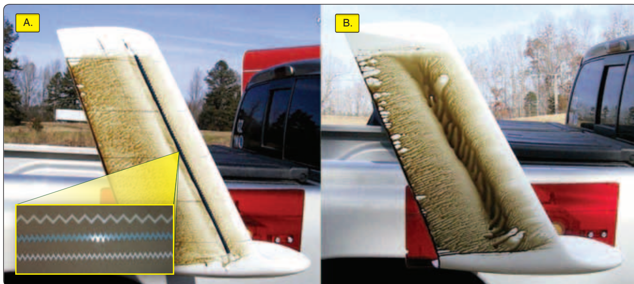
Figure 3-10. Glider wing on the left shows the airflow with a turbulator installed and the glider wing on the right shows how the airflow is disturbed without the turbulator installed.
