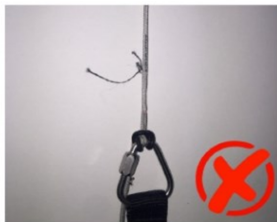
Fig. 4: Open thread-ends pulled out –NOT OK
