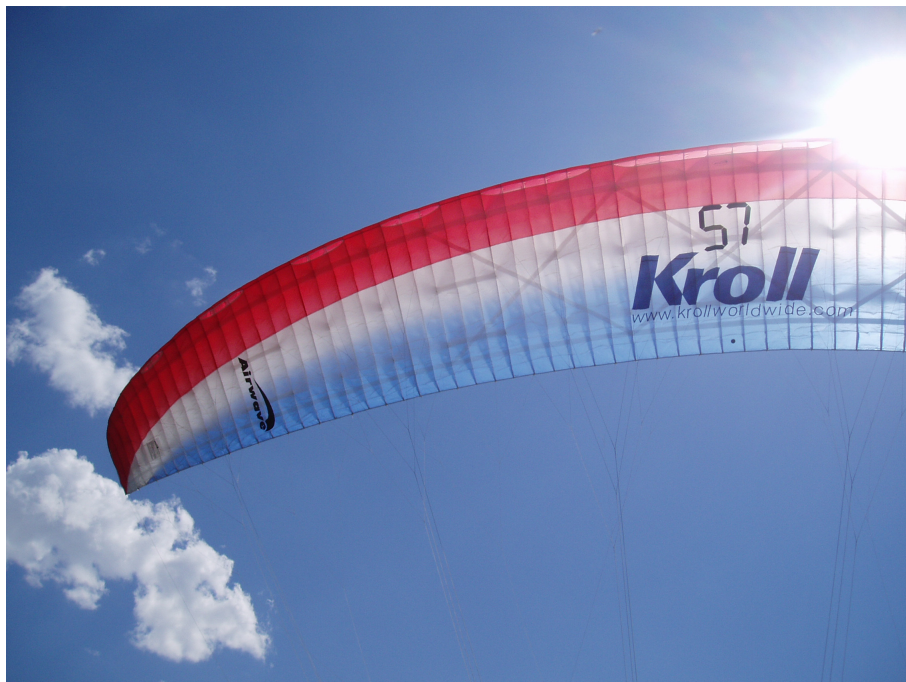
Airwave's latest Magic FR high aspect ratio competition prototype! Note X bracing.
