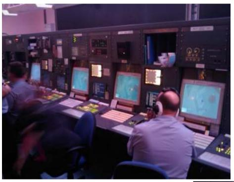
Above that screen can be seen the weather station data readout, there are also radios further along. The bad weather did have one positive benefit that day: the two incoming planes would require a 'talkdown' service because the visibility was too low VFR. for **Talkdown** involves other two screens (more basic than the others) with a sloping elevation line displayed above a runway alignment line; again the radar data is superimposed over the top.
