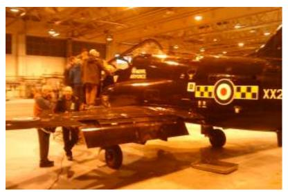
Notice the slot between the wing and the flap, this, we were told, is to improve performance close to the stall in tight manoeuvres. Two more pilots came downstairs and talked to us about 100 squadron's usual operations; these generally involve either pilot training, or providing targets for Typhoons during aggressor training. The distinctive skull and crossbones logo is 100 Squadron's highly coveted motif.
